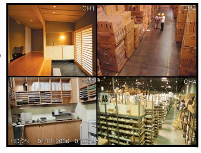
If a camera is not detected, or the Camera is in COVERT MODE, the associated portion of the QUAD or MULTI screen will display a BLUE SCREEN.
